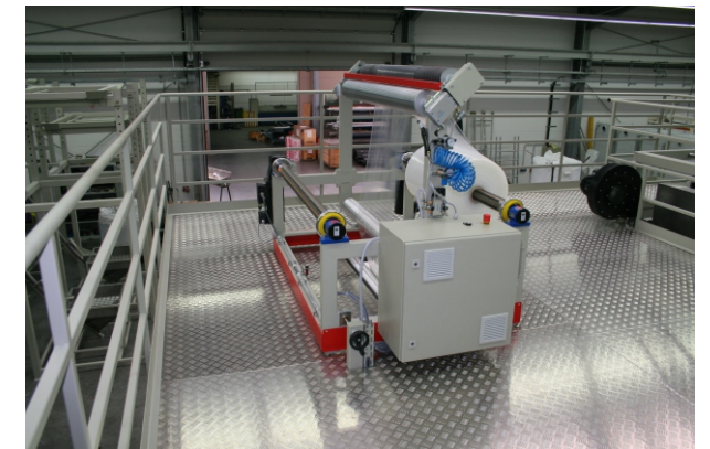
Unrolling from a stage with integrated haul-off
