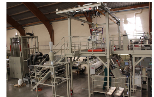
Unrolling from a platform with an integrated gantry crane
