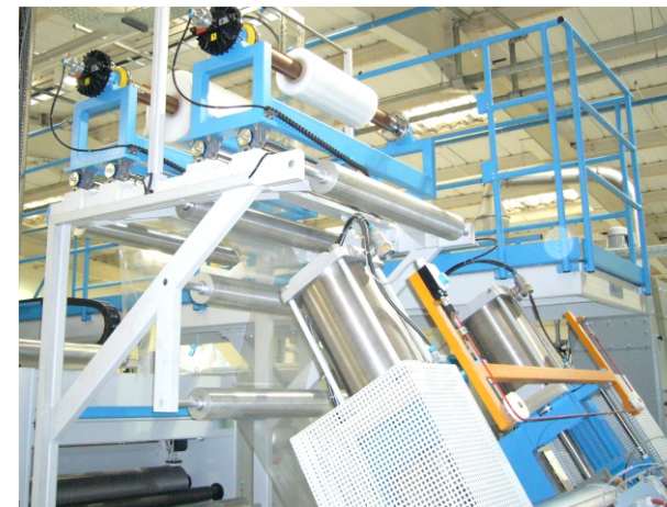
Unwind directly above the calender with side platform
